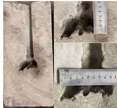
Figure 13. Reaming effect at a nozzle angle of 30° and spacing of 15 mm.
