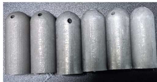
Figure 9. 3D-printed spray head.
