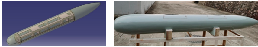
Figure 10. Drag reduction experimental model for superhydrophobic surface coating on underwater vehicle hull.
