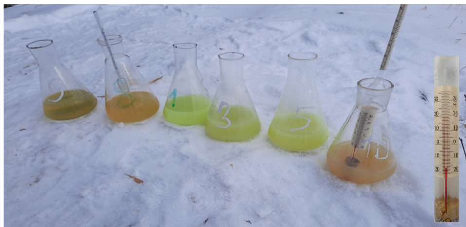
Figure 8. Clouded or jellied samples of biodiesel–diesel blends at -20\text{ }^{\circ}\text{C} (an explanation of the numbers is shown in Table 2).
