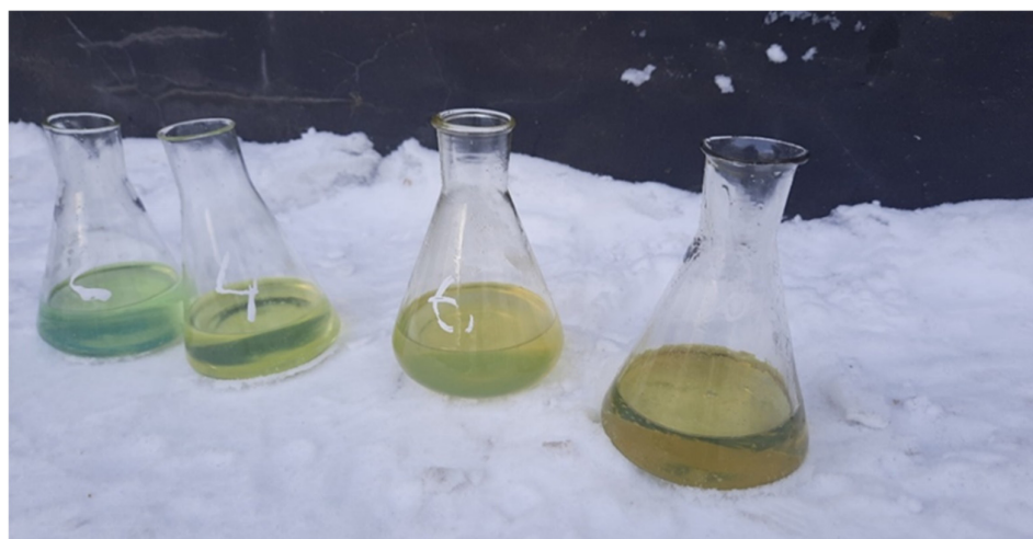
Figure 9. Samples of biodiesel–diesel blends retaining fluidity at -20\text{ }^{\circ}\text{C} (an explanation of the numbers is shown in Table 2).
