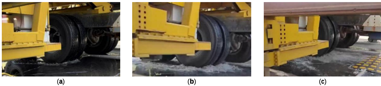
Figure 15. Instantaneous states of tire-water-pavement coupling interaction with different water depths in field tests: (a) 10 mm; (b) 15 mm; (c) 20 mm.
