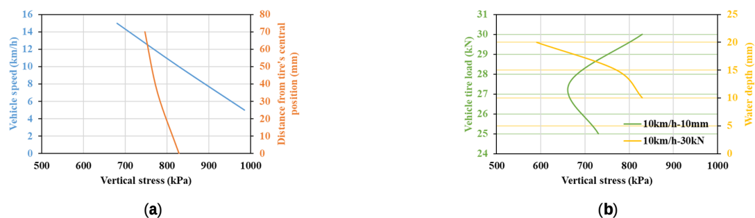
Figure 18. Variation in contact vertical stress with variable parameters in field tests: (a) Speed (30 kN-10 mm); (b) Tire load (10 km/h-10 mm) and water depth (10 km/h-30 kN).
