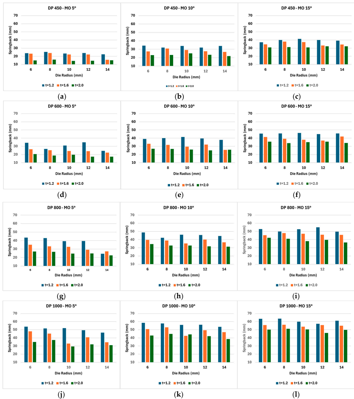
Figure 5. Comprehensive experimental springback data for 180 forming scenarios, categorized by material grade and mold opening angle (MO): (a–c) DP450, (d–f) DP600, (g–i) DP800, and (j–l) DP1000. All charts are standardized to a 10–70 mm scale for direct comparison.
