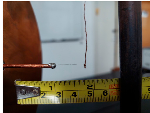
Figure 11. Image of the distance between the textile thread and the tip of the antenna after the thread has detached.
