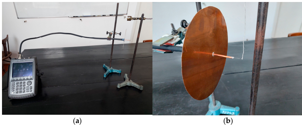
Figure 9. Pictures of the experimental arrangement for proving the microwave dielectrophoresis force: general view (a) and details with the antenna and pendulum (b).
