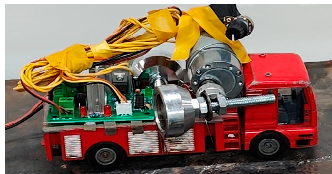
Figure 4. Moving Load Application Device.
