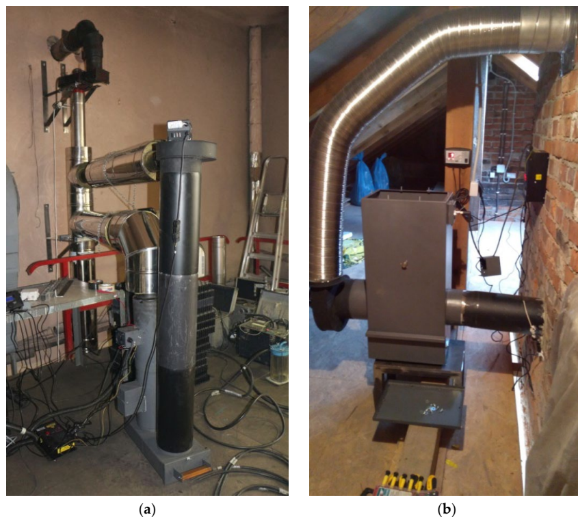
Figure A4. Pictures of the ESP during operation; (a) laboratory testing, (b) field testing.
