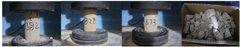
Figure 3. Failure modes of similar materials.
