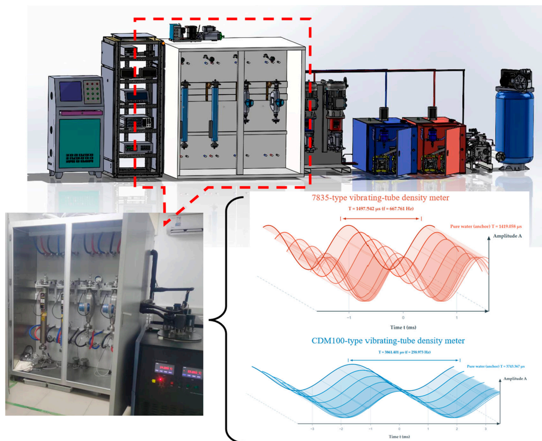
Figure 4. Calibration system in NIM. The red dashed box marks the density meter under test.
