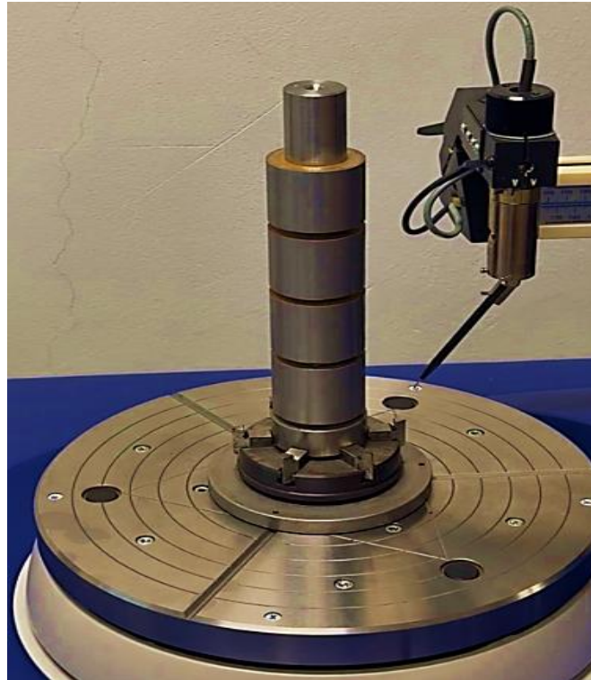
Figure 7. Taylor Hobson Talyrond 365 setup for cylindricity and concentricity measurement.
