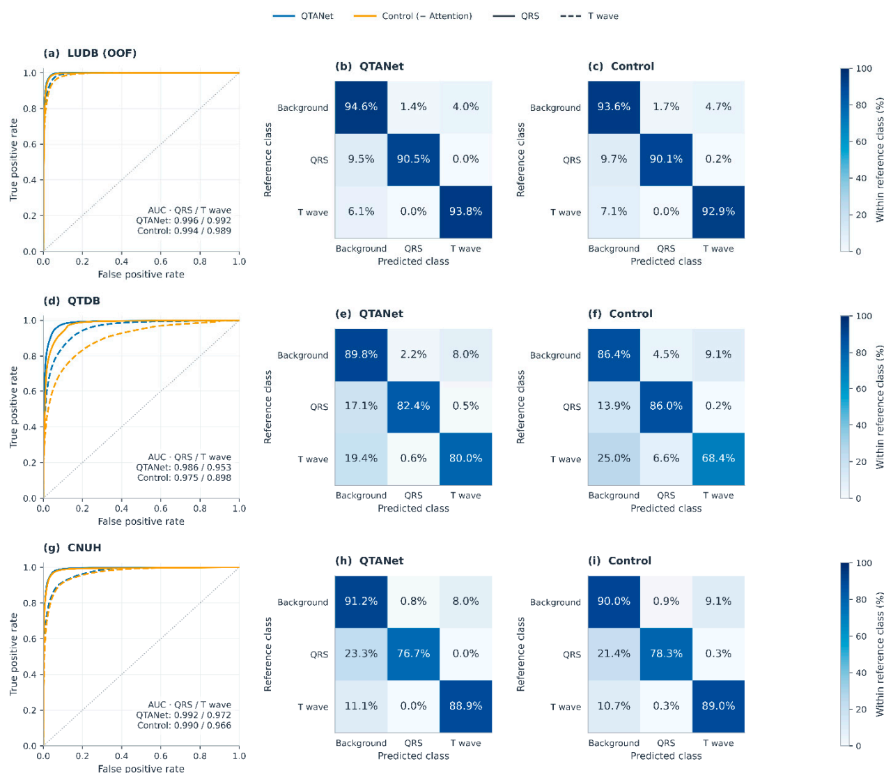
Figure 3. Frame-level waveform classification for QTANet and Control (–Attention). (a,d,g) ROC curves for QRS and T wave on LUDB (OOF), QTDB and CNUH, respectively; (b,c,e,f,h,i) the corresponding row-normalized confusion matrices. Solid and dashed curves denote QRS and T wave, respectively; colors distinguish models. Matrix entries are percentages within each reference class and may not sum to exactly 100% because of rounding. LUDB and CNUH use expert annotations; QTDB uses the automatic reference. The LUDB OOF panel is distinct from the fixed-test summary in Table 1.
