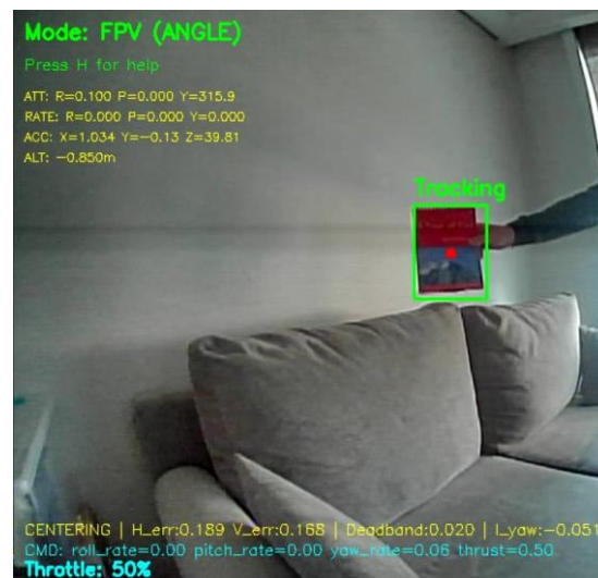
Figure 8. Representative frame from the yaw-only test-stand runs. The green bounding box marks the tracking region around a target object.
