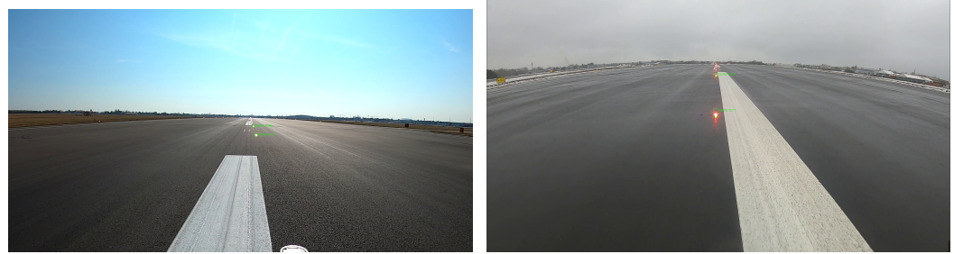
Figure 4. Representative output visualizations from the inspection prototype: a detected runway or taxiway light in a daytime frame ( left ) and colour-coded light detections along an airfield marking under reflective conditions ( right ).
