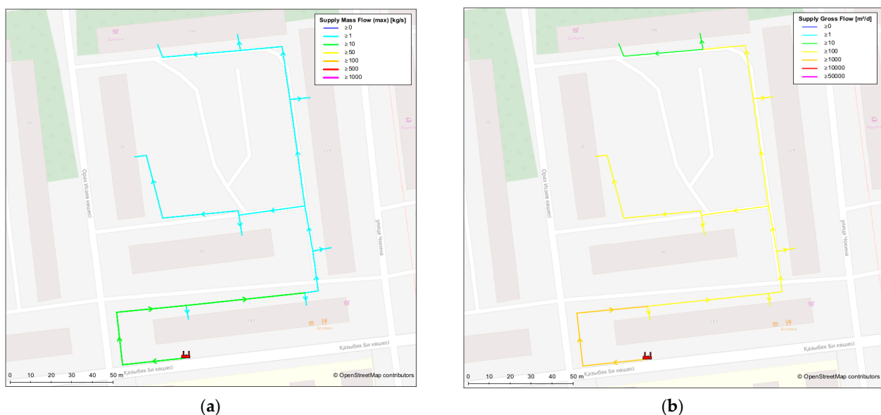
Figure 10. Fluidit Heat drawing states of the modeled network: maximum supply mass flows in kg/s displayed using the “Supply Mass Flow” view (a) and daily gross supply flows in m 3 /d displayed using the “Supply Gross Flow” view (b). Arrowheads indicate flow direction, and line colors
