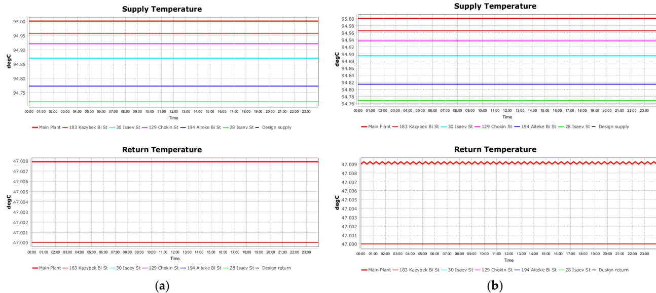
Figure 16. Time profiles of supply and return temperatures (°C) at the main plant and monitored consumer nodes for the baseline (a) and 120% heat demand (b) scenarios. The design supply and return temperatures are included as reference lines. Some curves and reference lines overlap at the displayed scale.
