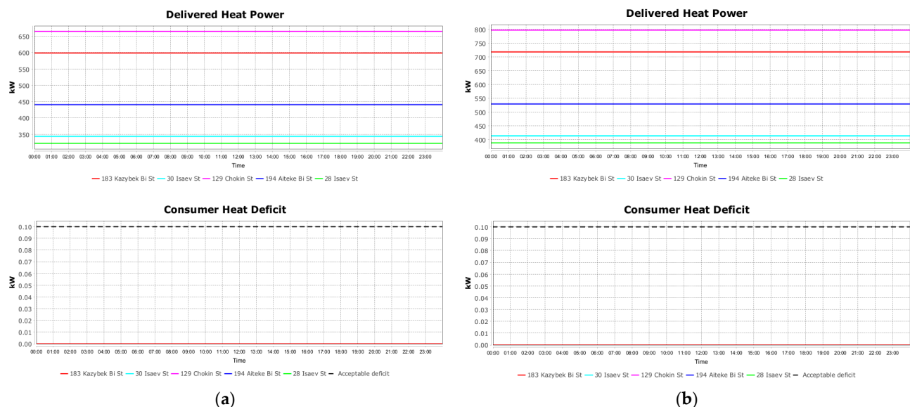
Figure 17. Time profiles of delivered thermal power and consumer heat deficit (kW) at the monitored consumer nodes for the baseline (a) and 120% heat demand (b) scenarios. The dashed black line in the heat deficit plots indicates the acceptable deficit threshold. The deficit curves overlap at zero.
