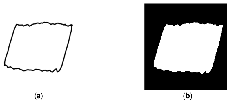
Figure 9. Comparison of dynamometer cards before and after processing: (a) Unprocessed dynamometer cards; (b) Processed dynamometer cards.
