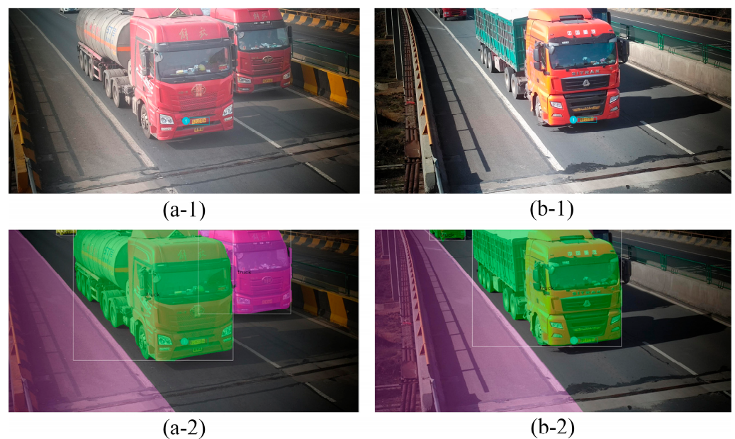
Figure 5. Vehicle instance-detection results in multi-vehicle scenes. (a-1,b-1), different vehicles to be detected; (a-2,b-2), detected result.
