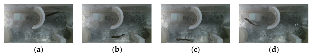
Figure 6. Swimming behavior of juvenile silver carp in island-type fishways (Case 3). (a) t_0 (b) t_0 + 1.93 s (c) t_0 + 3.10 s (d) t_0 + 5.57 s.
