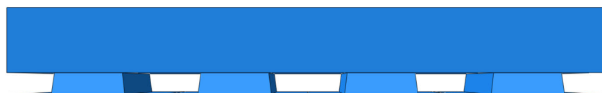
Figure 18. Model of the mass block assembly connected by molded pulp structural cells.
