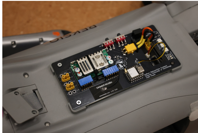
Figure 3. The custom power management and interface board.
