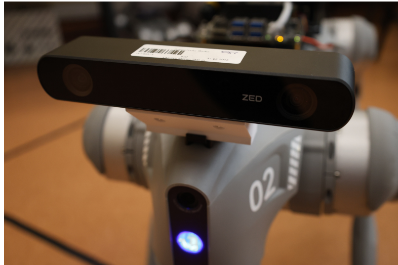
Figure 6. The Stereolabs ZED2i stereo camera utilized for target detection and 3D localization.
