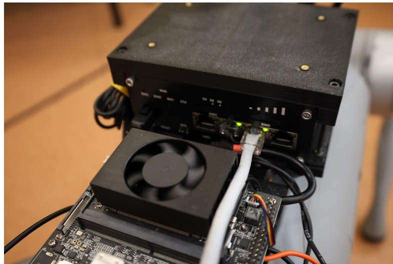
Figure 5. The Teltonika RUTM11 industrial router providing GNSS and dual-mode networking.
