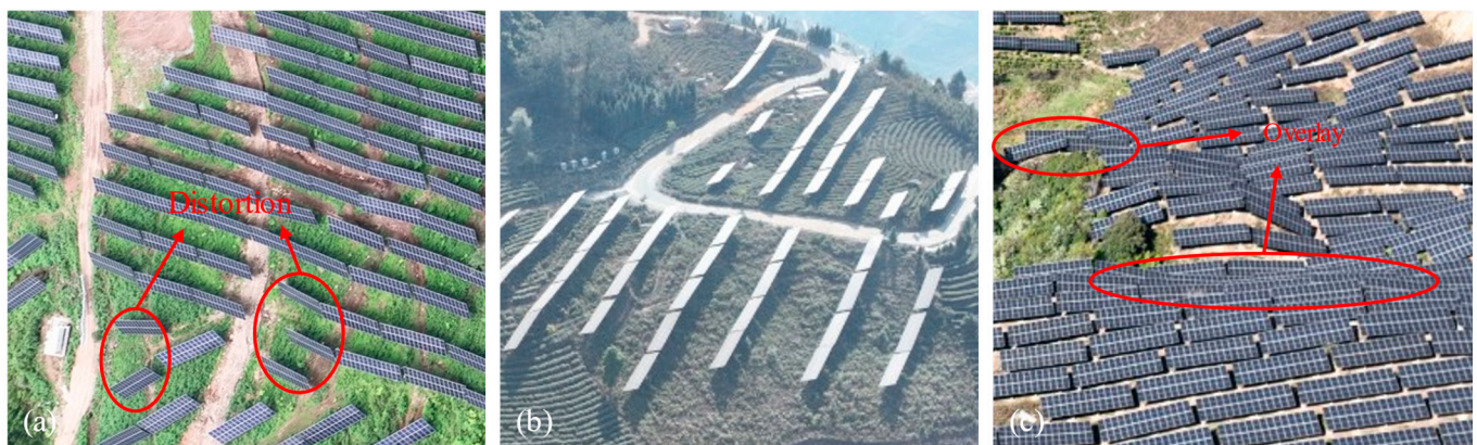
Figure 1. Imaging conditions in the acquired UAV data. (a) Perspective distortion; (b) strong specular reflection; (c) array overlap and boundary ambiguity.
