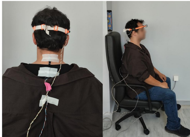
Figure 5. The experimental setup demonstrating the anatomical placement of the dual-node sensor array on the cranial vertex and the C7-T1 region. The subject maintains a neutral, fully supported seated posture ( 0^\circ cervical flexion) during the T_0 baseline calibration phase. This position establishes the initial syntropic stability, supporting the actual anatomical head weight of \sim 5 kg prior to workload induction. (Note: Facial features have been obscured to maintain subject anonymity in accordance with ethical guidelines.)
