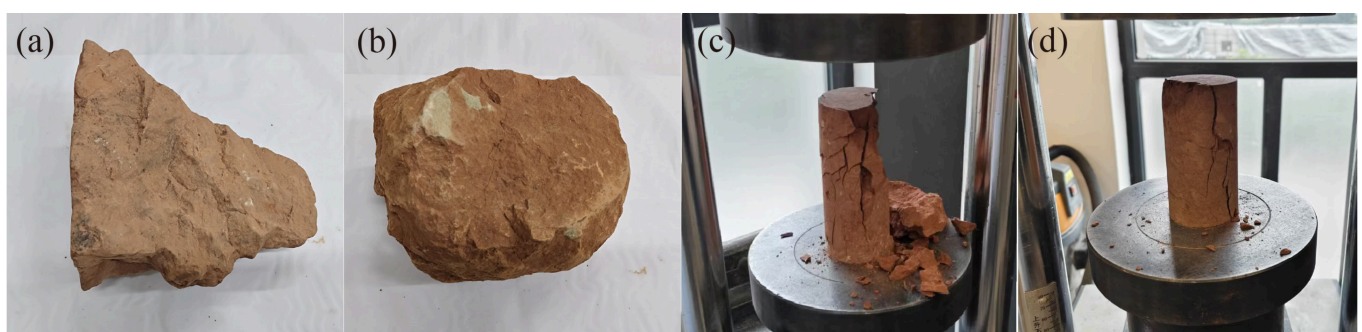
Figure 3. Representative macroscopic appearance and typical failure characteristics of red-bed soft rocks during laboratory testing: (a) representative rock block from Sampling Site ①; (b) representative rock block from Sampling Site ②; (c) fragmentation and spalling failure after mechanical testing; (d) cracking and splitting failure after mechanical testing.
