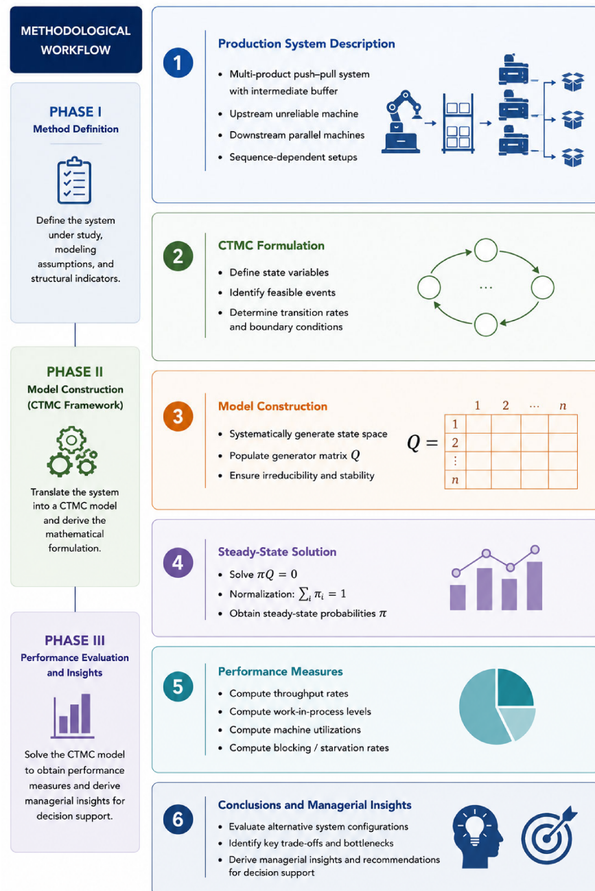
Figure 1. Methodological framework for the CTMC-based modeling and performance evaluation of the proposed multi-product push–pull production system.
