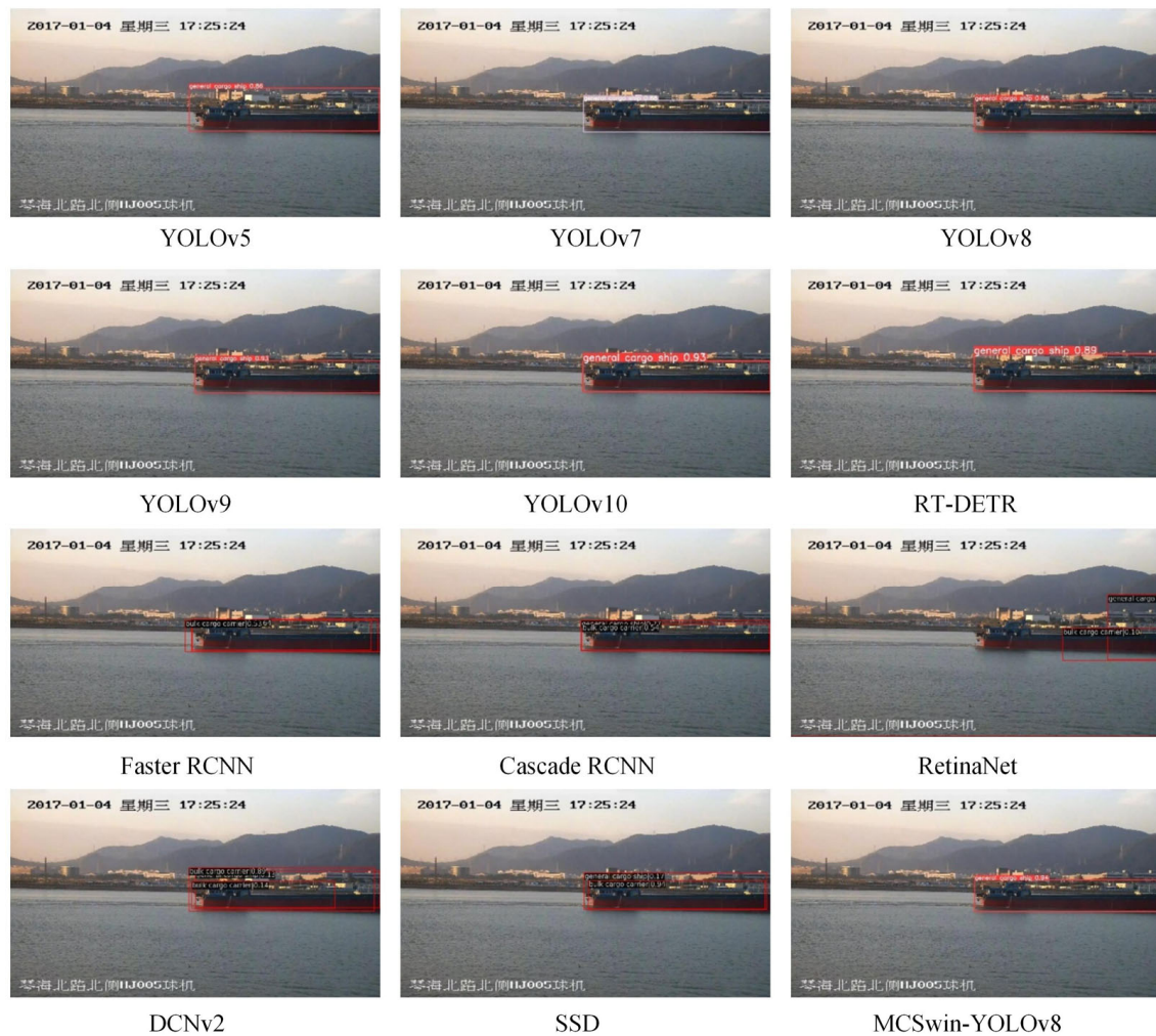
Figure 13. Visual comparison of different detectors in a single-target scene from the SeaShips test set. The non-English text is an embedded timestamp/source watermark from the original dataset image; it is not an annotation or model prediction.
