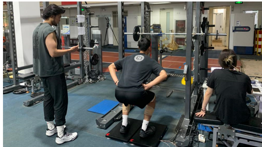
Figure 1. CMJ test execution. An athlete performs a maximal countermovement jump on a force plate; ground-reaction forces are recorded by the data-acquisition laptop.
