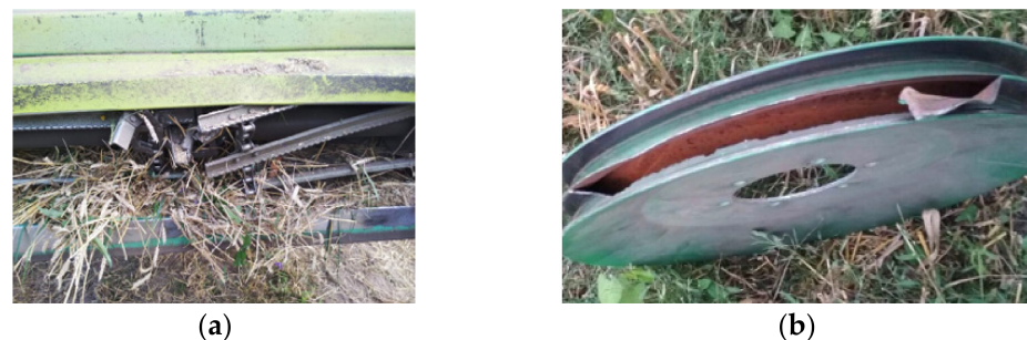
Figure 5. (a) Feeding device chain fracture [5], (b) Header drive wheel damage [5].
