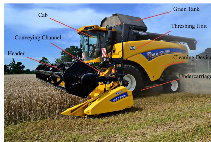
Figure 4. Structure and major components of a typical combine harvester.
