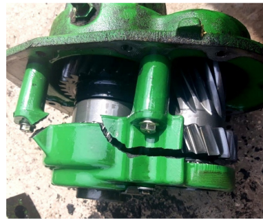
Figure 8. Break in the gearbox cover [5].
