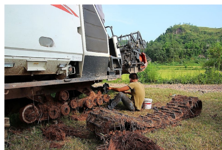
Figure 9. Track disassembly for field repair (illustrative photograph).
