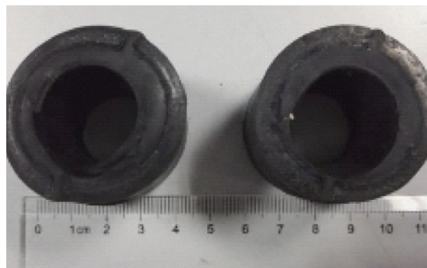
Figure 7. Rubber bearing wear diagram [65].
