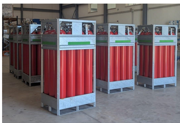
Figure 15. Bundles of high-pressure gas cylinders awaiting interconnection in the prototype CAES system. Some bundles are partially hidden from view.
