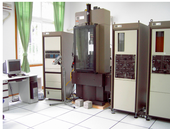
Figure 5. The MTS815 electro-hydraulic servo rock testing system.
