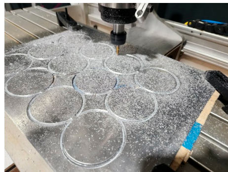
Figure 5. Aluminum face sheets fabricated by the CNC machining process.
