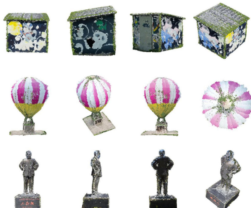
Figure 3. This figure illustrates the high-fidelity object reconstruction results produced by our proposed four-stage enhanced NeRF pipeline. Multi-view renderings of the house ( top row ), balloon ( middle row ) and sculpture ( bottom row ) are presented. These outcomes validate that our method can capture fine geometric structures and accurate surface textures from monocular video input, providing a crucial foundation for the subsequent point cloud completion stage.
