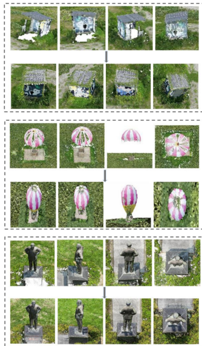
Figure 5. This figure presents the final results of our point-cloud completion pipeline achieved through registration and fusion. Multi-view renderings of the three target objects—house ( top ), balloon ( middle ), and sculpture ( bottom )—are shown; for each object, the upper row displays the model before completion, while the lower row shows the same model after completion. Comparing the two, it is evident that the completed models recovered the geometric information missing in the initial fragments extracted from the large-scale scene, whether the loss was caused by occlusion or by inherent limitations of the reconstruction algorithm. Surface holes were effectively filled, leading to a marked increase in fidelity and overall quality. These results confirm the effectiveness of our registration workflow, which compensates for the well-known inability of large-scale reconstructions to capture fine local detail, and yields models of significantly higher practical and scientific value.
