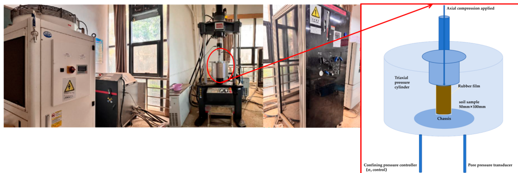
Figure 2. MTS servo hydraulic fatigue testing machine.
