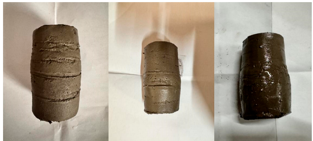
Figure 4. Failure mode of soil sample.
