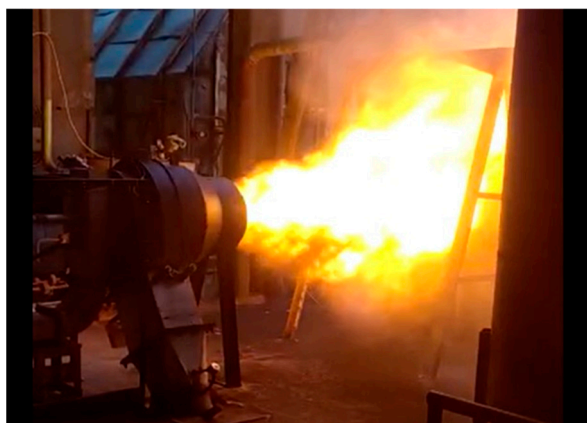
Figure 8. Flame extending up to 4 m at a coal feed rate of approximately 3000 kg/h.
