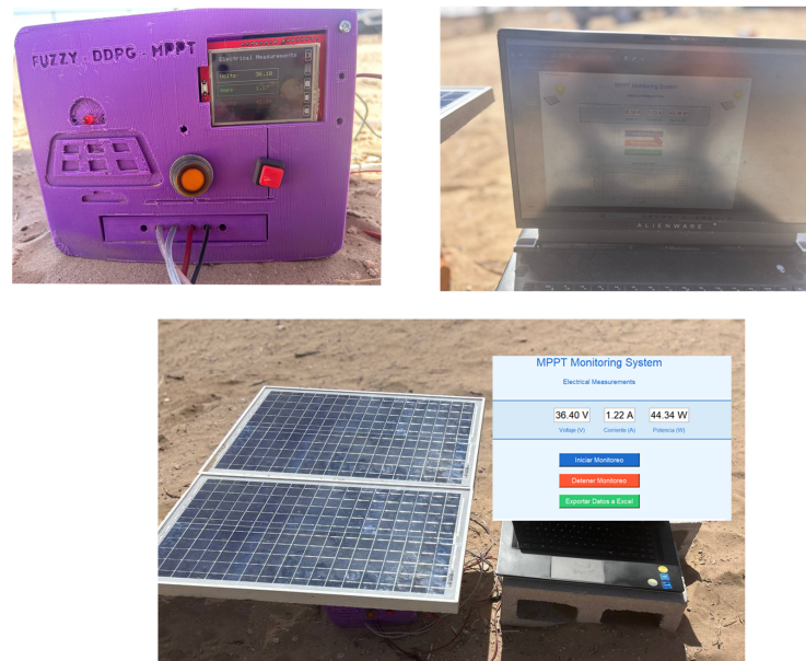
Figure 15. Physical implementation of the MPPT system. The image shows the panels under partial shading conditions, along with the power electronics, control hardware, and battery enclosure.
