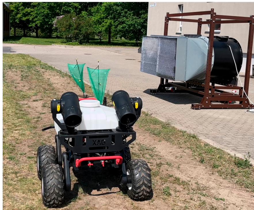
Figure 8. The real view of orchard spray experiments with a robot sprayer.
