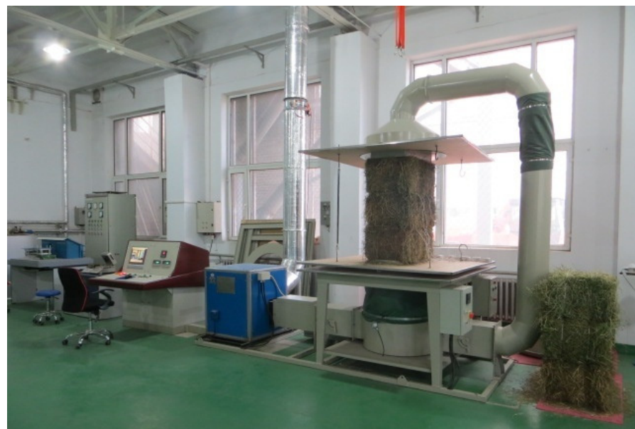
Figure 1. Field diagram of the hay bale drying test.
