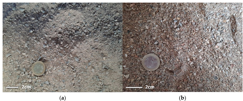
Figure 6. Aggregates used in this study: (a) natural calcareous; (b) CDW.
