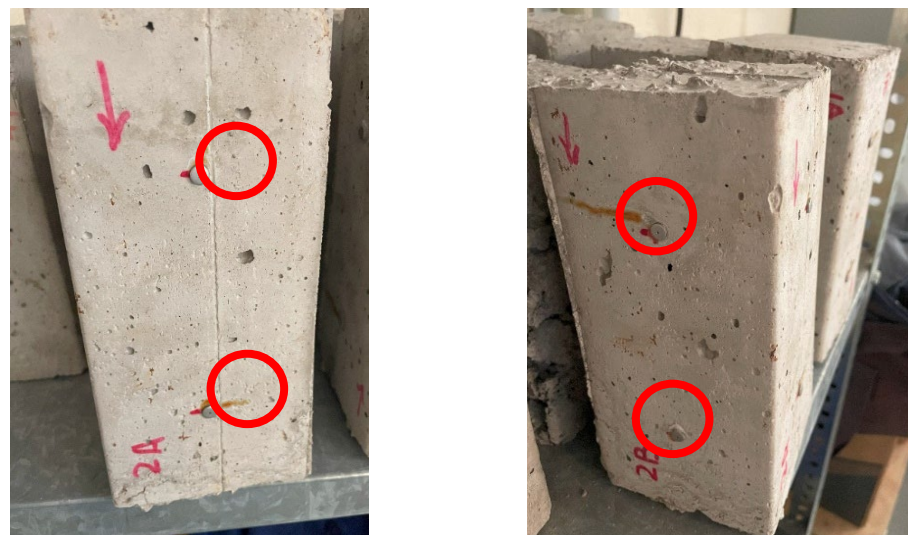
Figure 4. Concrete samples for shrinkage measurements. Reference points marked with red circles.
