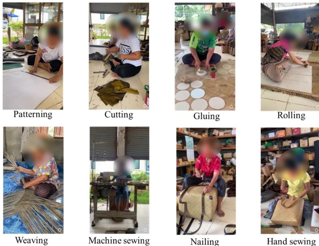
Figure 1. The stage processing and postures of shoulder bag production.
