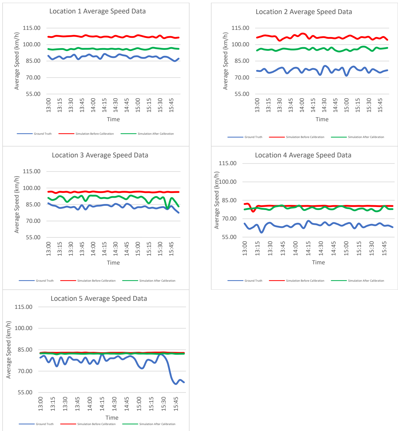
Figure 7. Average speed comparison of ground truth and simulation results before and after the calibration process.
