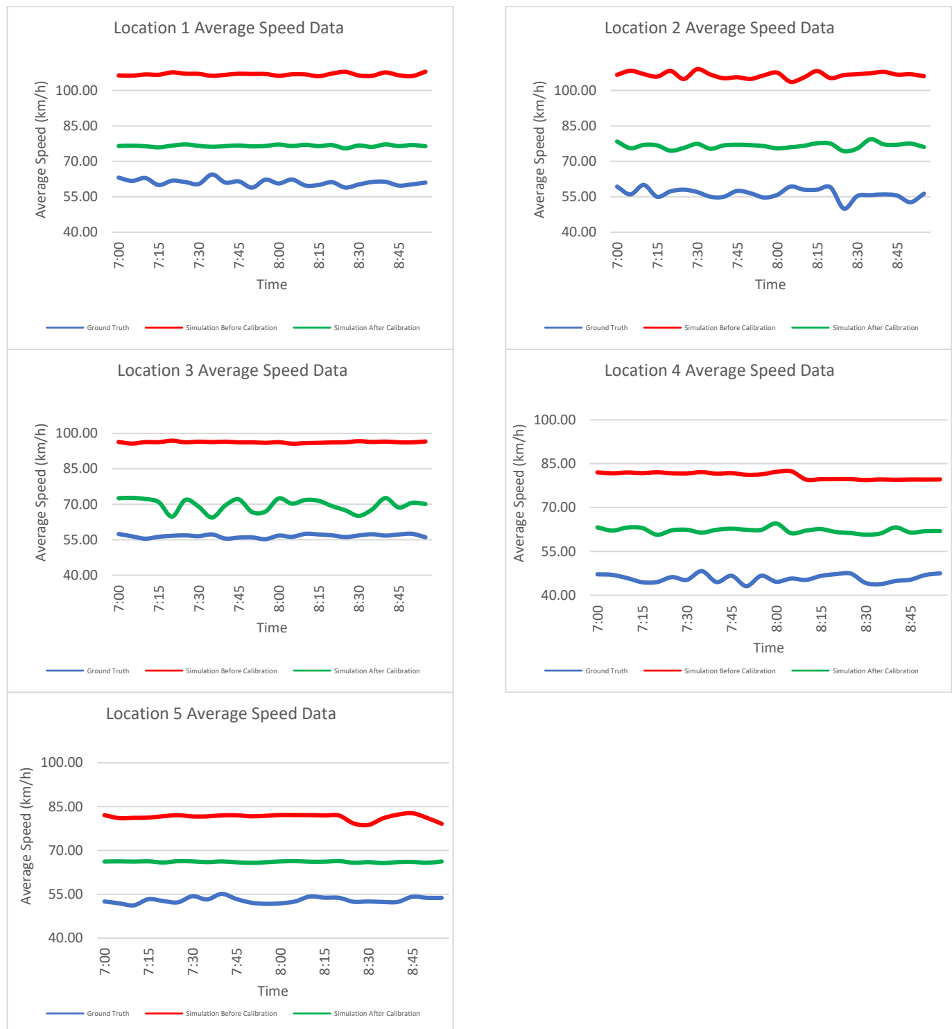
Figure 8. Average speed comparison of ground truth and simulation results before and after implementing calibrated parameters in the validation process.
