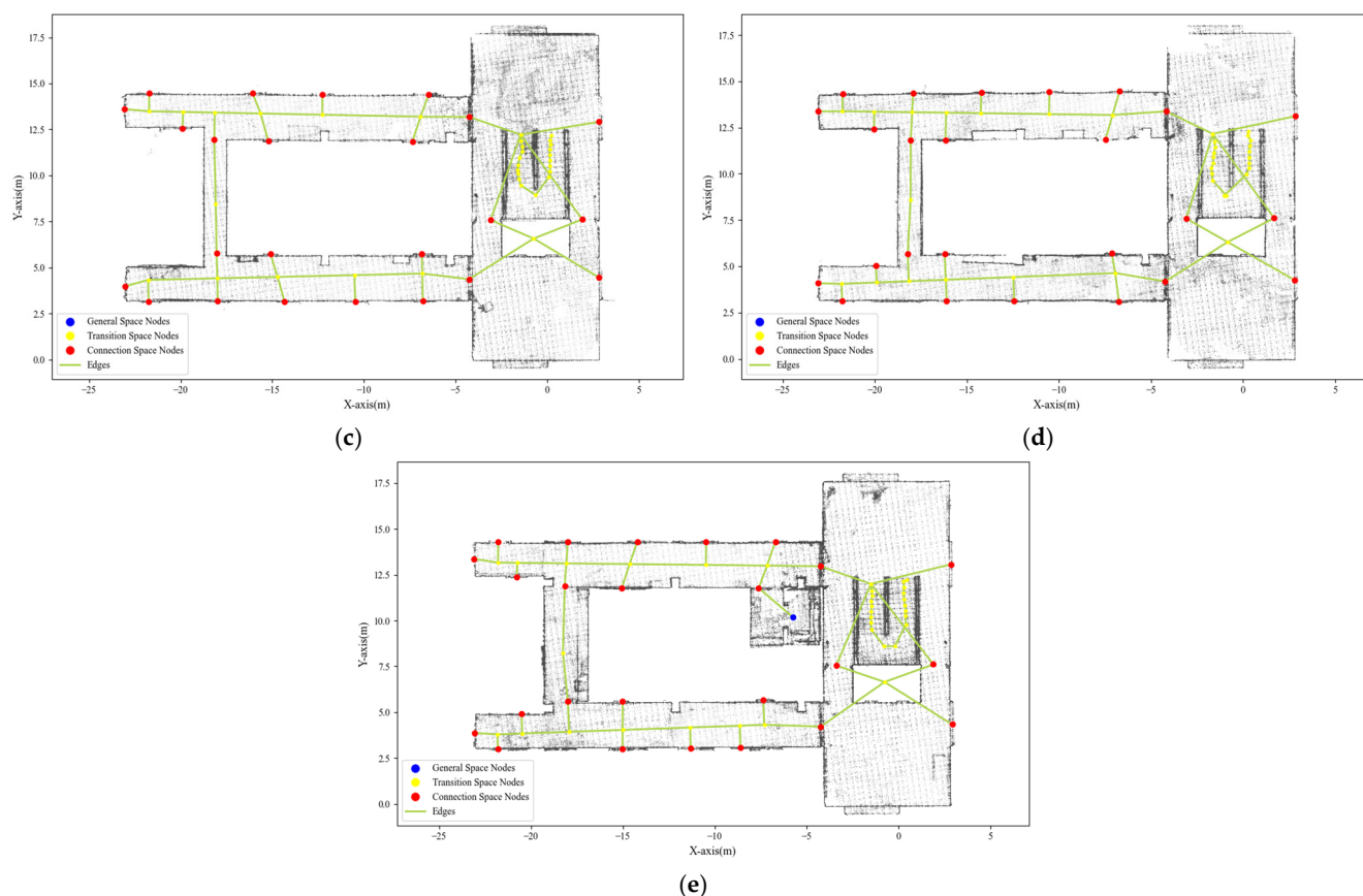
Figure 15. The results of the extracted indoor navigation network with self-collected dataset: (a) floor 0, (b) floor 1, (c) floor 2, and (d) floor 3, (e) floor 4.
