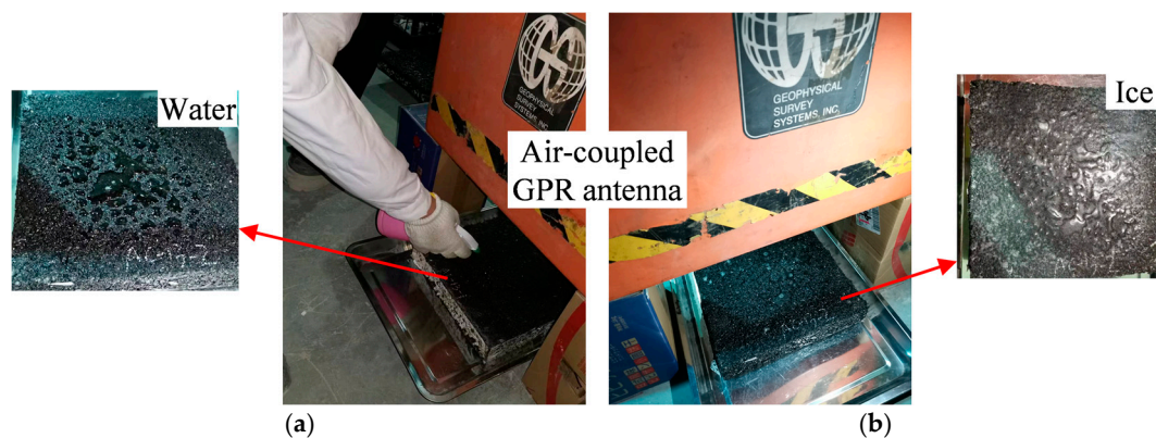
Figure 5. AC-13 slab with different surface states detected by GPR: (a) water, (b) ice.
