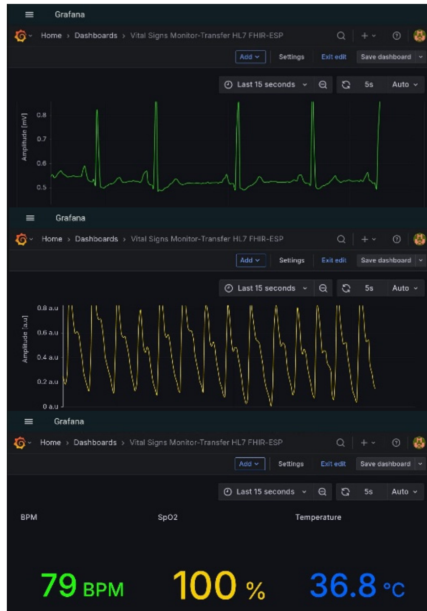
Figure 10. Panels for monitoring biomedical data transmitted via the HL7 FHIR mobile interface on mobile devices.
