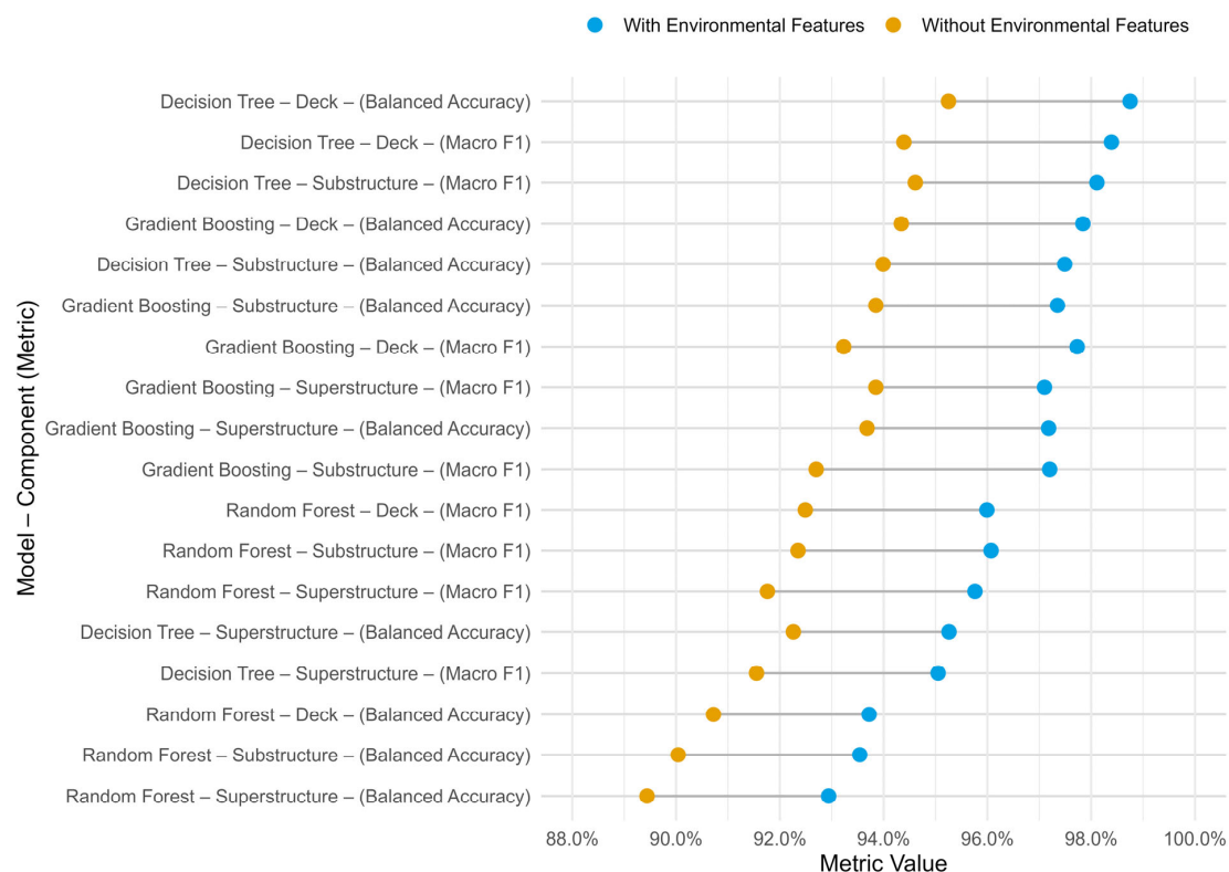
Figure 4. Performance gains achieved by incorporating environmental variables into Decision Tree (DT), Random Forest (RF), and Gradient Boosting (GB) models. Improvements are shown across deck, superstructure, and substructure components for three metrics (Balanced Accuracy, MCC, and Macro F1).
