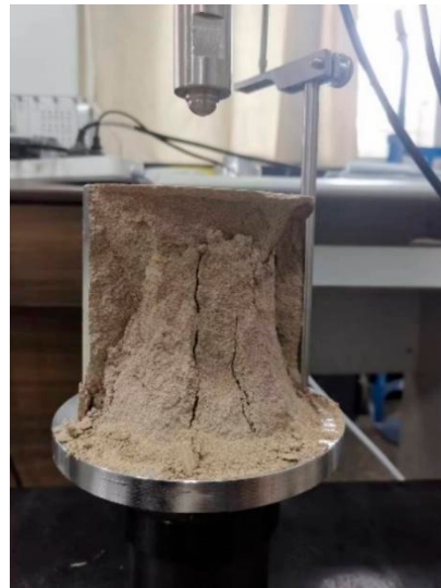
Figure 8. Final failure form of the sample.
