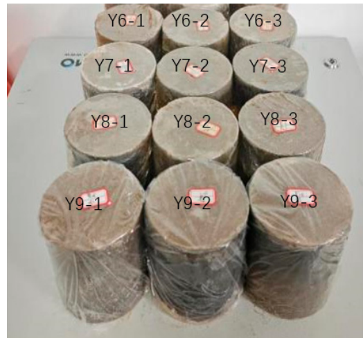
Figure 3. Cement-modified aeolian sand sample.
