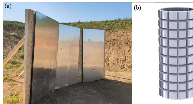
Figure 2. (a) Experimental setup for detonation of a steel-cased cylindrical charge at 500 mm above the ground in front of three panels; (b) steel casing with grenade-like pattern.
