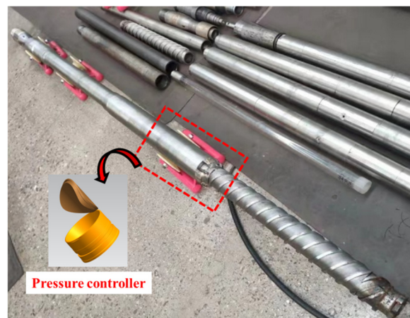
Figure 3. Prototype of deep in situ pressure coring tools.
