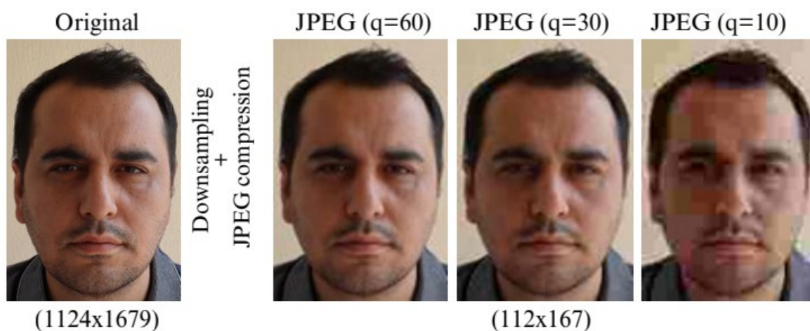
Figure 5. Downsampling followed by JPEG compression. (Image sizes: original \rightarrow 358 KB, q = 60 \rightarrow 3.04 KB, q = 30 \rightarrow 2.16 KB, q = 10 \rightarrow 1.43 KB).
