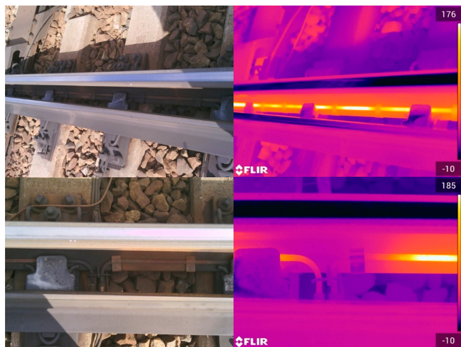
Figure 4. Resistance heater: on the left are photos of the heater, and on the right are thermograms.
