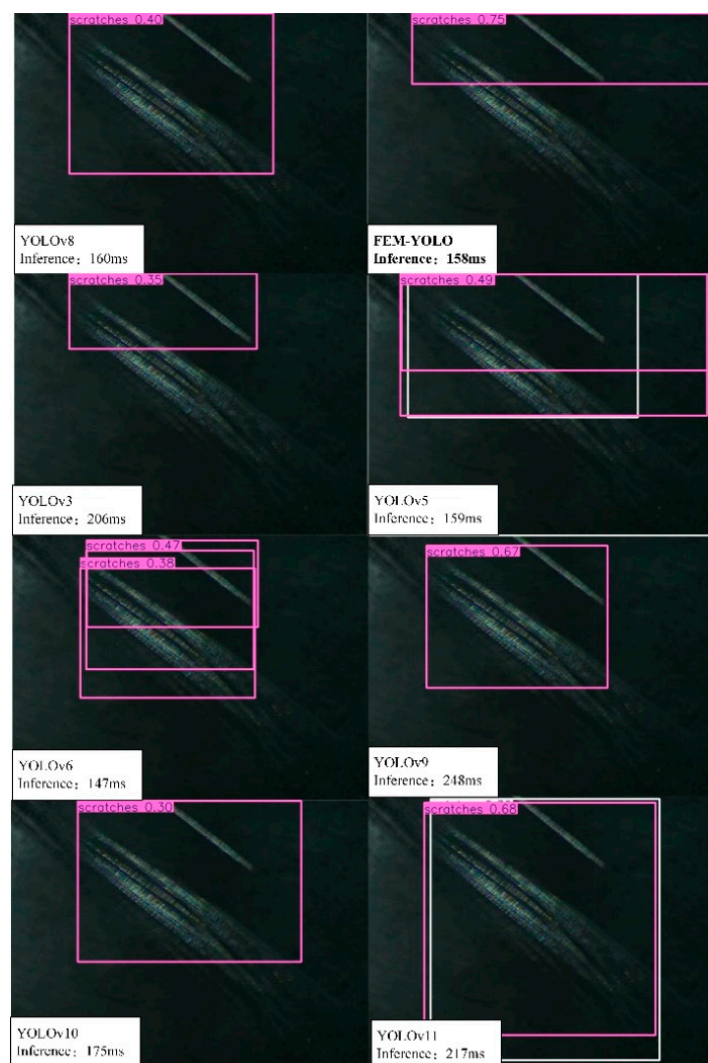
Figure 12. Model inference speed comparison results.
