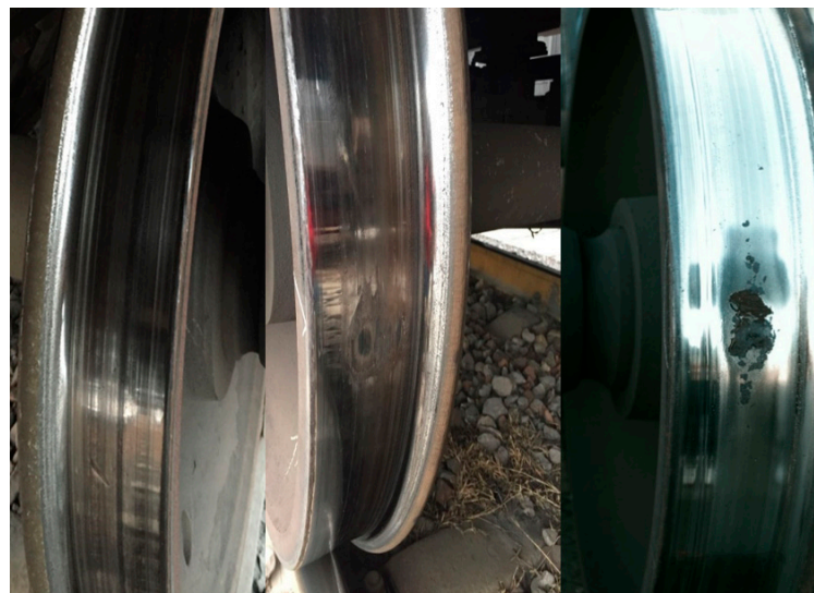
Figure 1. Image of wheelset tread defects. There are three main types of defects—pit, bruise, and peel.
