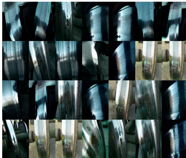
Figure 3. Wheel tread defect images generated by StyleGAN3.
